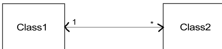
Figure 4.9 Bidirectional Association and Target/Source Multiplicity
