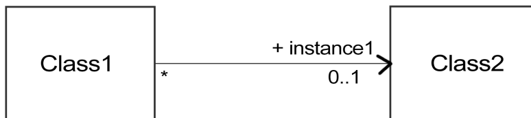
Figure 4.8 Unidirectional Association with Property Name, Target Multiplicity, and Source Multiplicity
