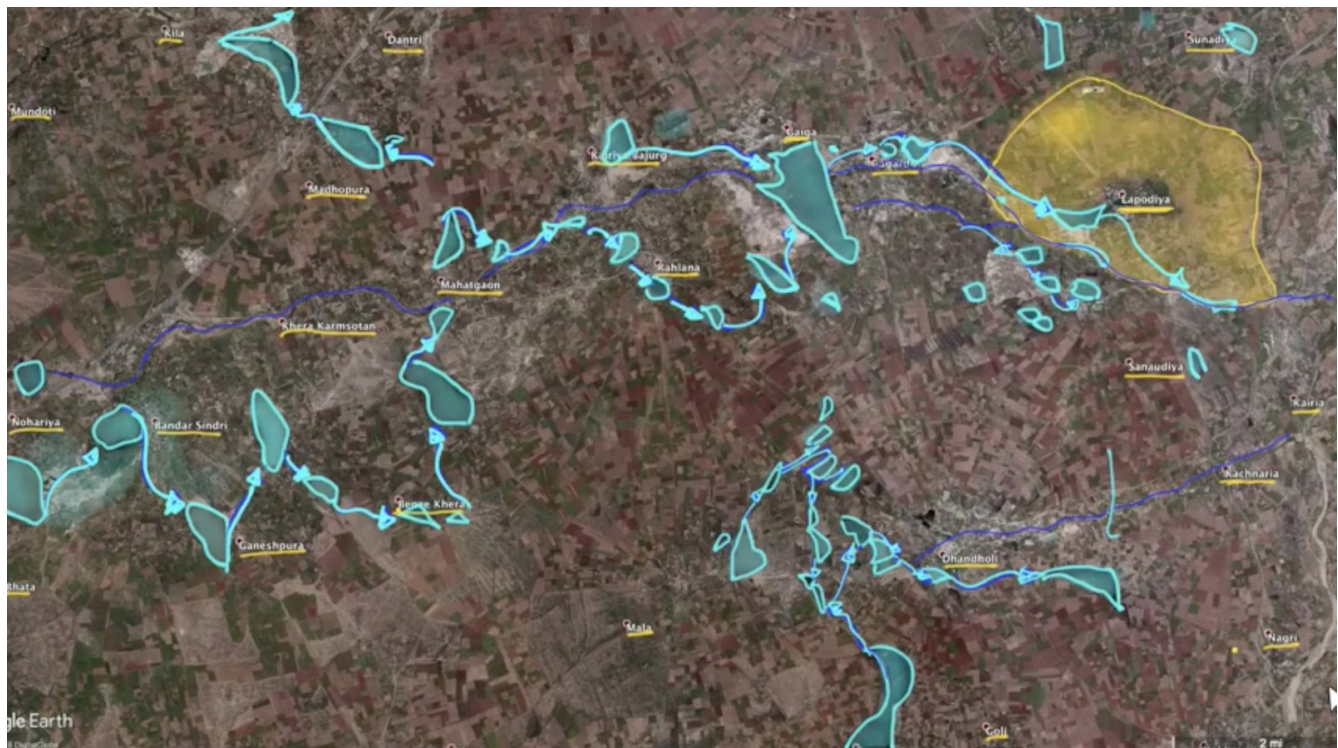
Figure 54 Interconnected ponds overflow from one to the next between multiple villages within a watershed.
