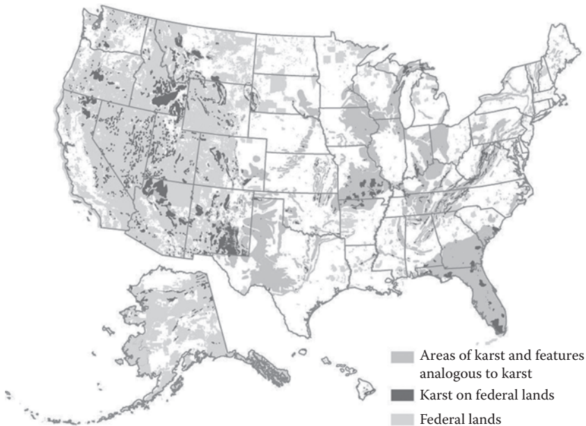
FIGURE 5.1 Locations of karst geology in the United States. These areas are prone to caves and subterranean streams and often require special consideration during forest management. (Reprinted from the National Cave and Karst Institute, USDI National Park Service.)
